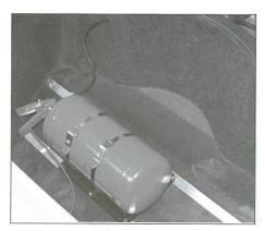
TIP 1: I used beveled bolts and came up from the bottom of the bottle assembly with nyloc nuts on top. This allows the aluminum frame to sit flush on the trunk floor.
