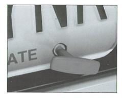
license plate. You will also need to make these bottom right holes big enough for the ENTIRE metal part of the handle to go through. The threads only go up 1/2" up the handle. It's just enough length to mount directly to the fiberglass body of the car.
