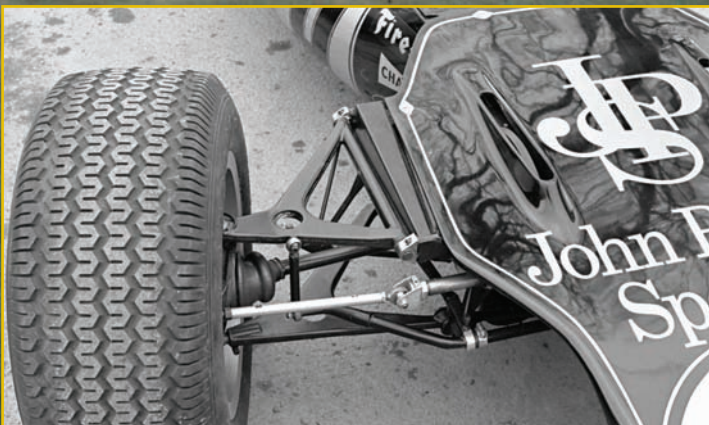
Front right rising-rate double-wishbone suspension.
