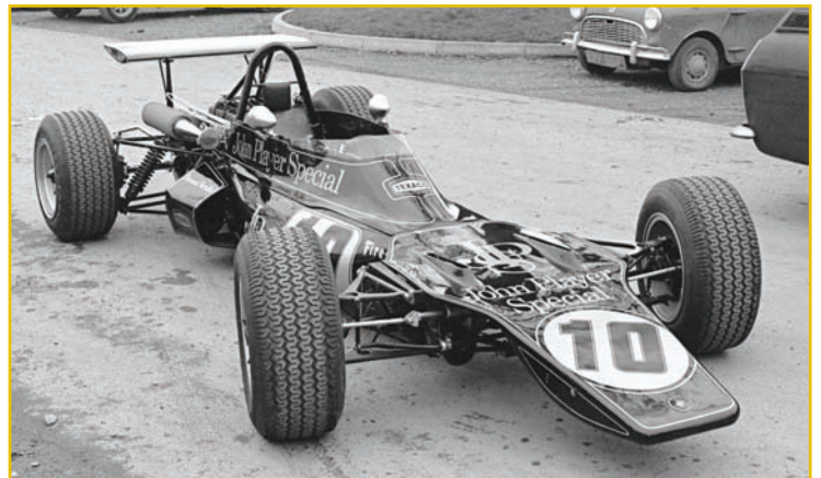
Built on a monocoque chassis with spaceframe cradle for the engine, the JPS 73 was a sophisticated design that never realised its potential.
