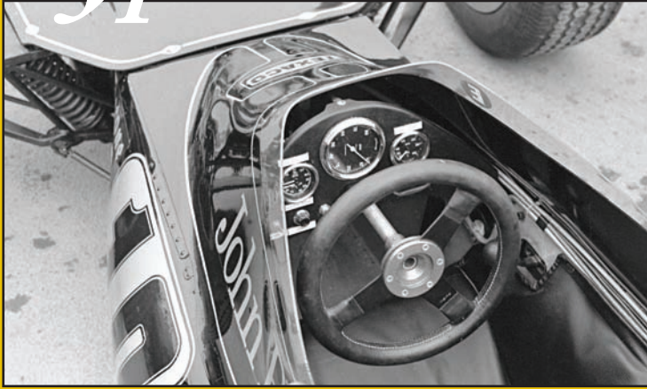
Three-spoke wheel, right-hand shift, central rev counter, the JPS 73 was an austere F3 cockpit.
